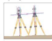
The biaxial level compensation mechanism has a wider adjusting range of  $\pm 6^{\circ}$  which is twice as wide, compared with previous models. This enables highly accurate measuring performance.
